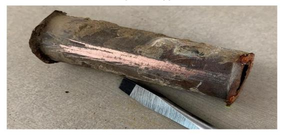
If your pipe appears metallic check to see if a magnet can stick to the pipe. If the magnet sticks, you have *GALVANIZED STEEL* pipe. See photo below:
